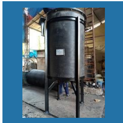
Spiral HDPE Reactor Vessel With Structure
